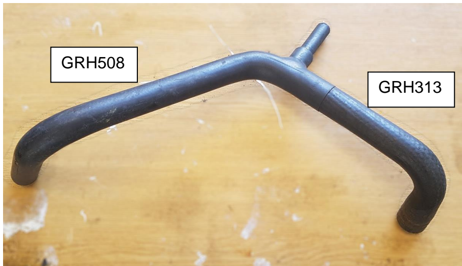
FIGURE 5: EARLY MIDGET HOSES LINKED TO RUN BEHIND ENGINE
