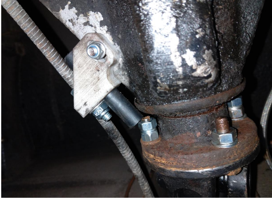
Figure 3: Bracket and sensor installed
